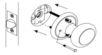
Specify hardware handing by standing on the outside of the house, room, hallway, or closet and note if the hinges are on the left or the right (it does not matter if the door swings in or swings out).
